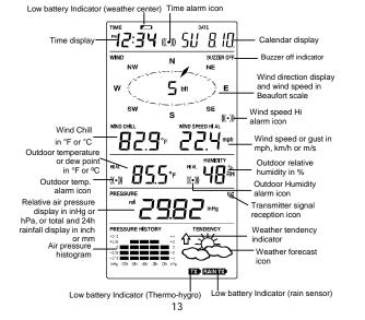
\* When the signal from the transmitter/ or Rain sensor is successfully received by the Weather Station, this icon will be switched on. (If not successful, the icon will not be shown on the LCD). User can therefore easily see whether the last reception was successful ("ON" icon) or not ("OFF" icon). On the other hand, the short blinking of the icon shows that a reception is being done at that time.
